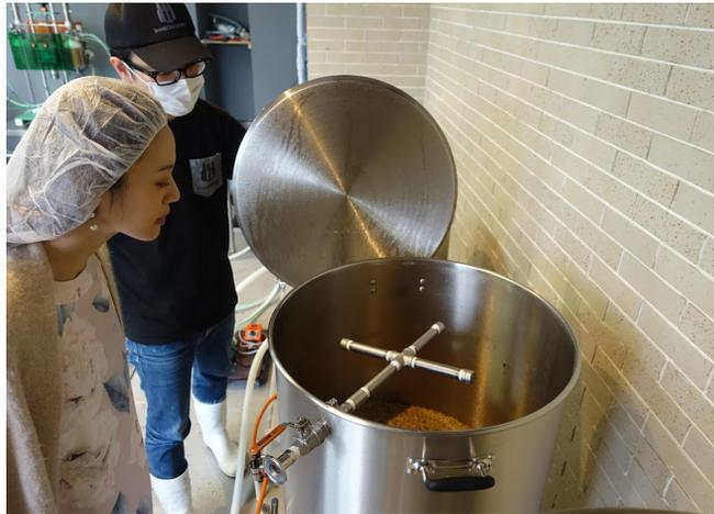
*Above, Daisuke shows a mash tun, where crushed grain (called grist) is mixed with hot water to create a sweet liquid (known as wort) that is used to make beer.*
