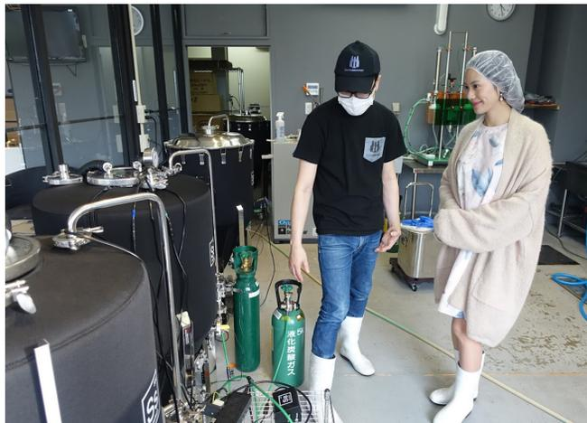
Daisuke explains that to start the fermentation, yeast is added during the filling of the vessel to convert the sugary wort into beer by producing alcohol and a wide range of flavors. It is necessary to keep the vessels at carefully controlled temperatures for the beer to ferment and mature properly.
